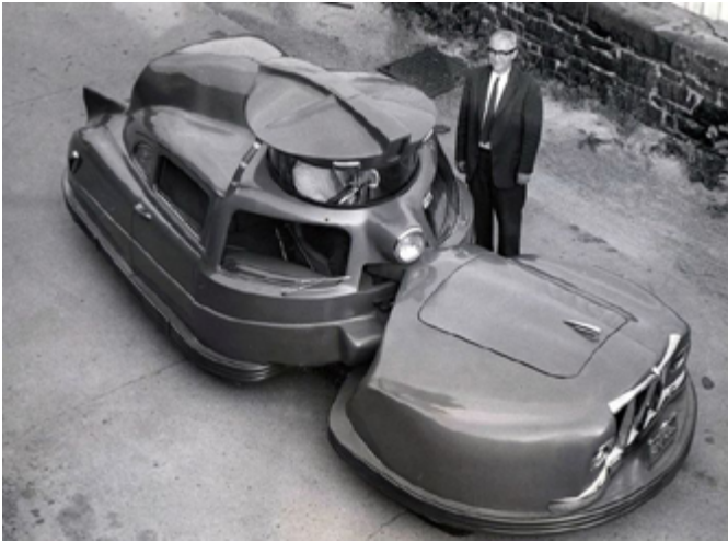
1958 Sir Vival. A two piece concept car created by Walter C. Jerome on mission to make the world's safest car.
